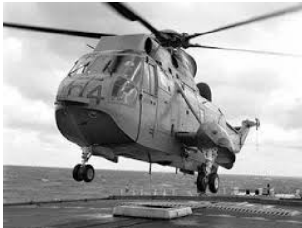
FIGURE 1.2: Helicopter being hauled down by a beartrap to land on the deck
