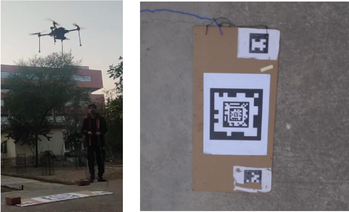
FIGURE 5.1: [Left]: UAV hovering above the marker to collect observations [Right]: Camera feed conversion
