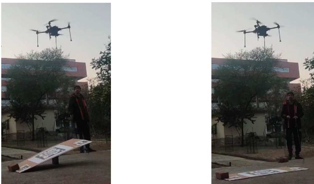
FIGURE 5.2: [Left]: Platform at 22° elevation from horizontal [Right]: Platform at 0° elevation from horizontal conversion
