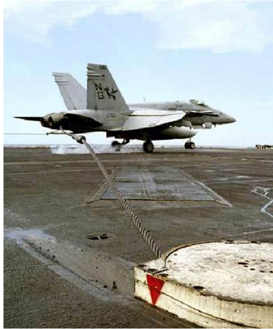
FIGURE 1.1: F/A-18C landing on aircraft carrier, showing arresting cable
