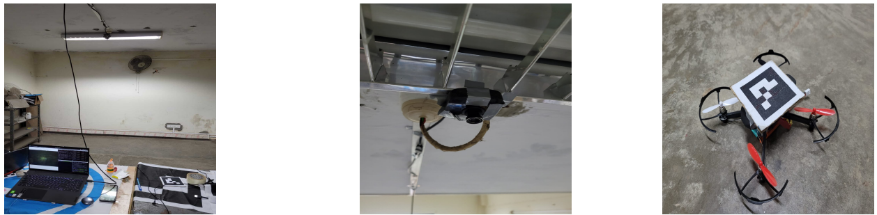
(a) Ground Station connected to the Camera (b) Camera duct taped to the ceiling (c) Drone with ArUco attached
